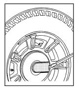
1. Remove the center cap by placing the flat end of the wheel wrench in the slot on the wheel and gently pry the center cap out.
